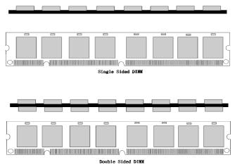
1. The DIMM slot has a " *Plastic Safety Tab*" and the DIMM memory module has a "Notched End", so the DIMM memory module can only fit in one direction.
