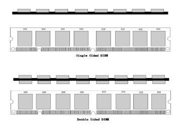
1. The DIMM slot has a " *Plastic Safety Tab*" and the DIMM memory module has a "Notched End", so the DIMM memory
