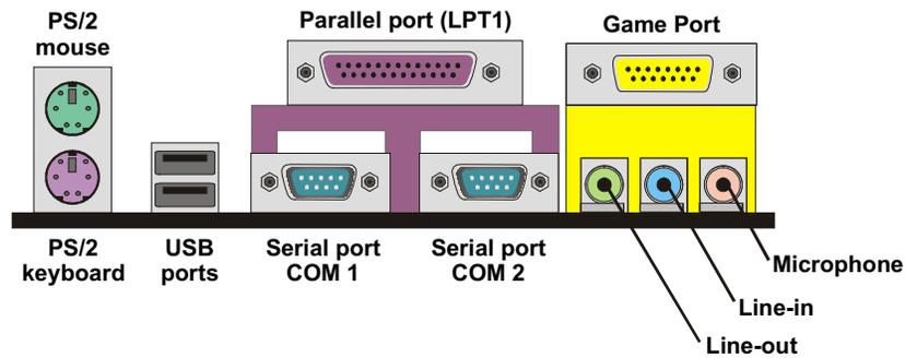
1. The PS/2 mouse port can be used by a PS/2 mouse or pointing device. The PS/2 keyboard port can be used by a PS/2 keyboard.
