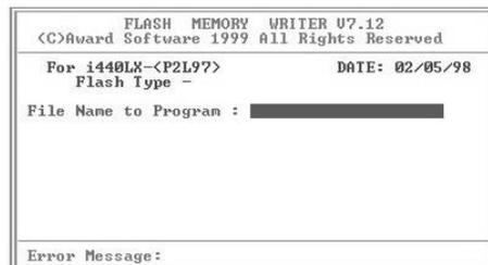
8. In the "File Name to Program" dialog box, type in the filename of the new BIOS and follow the onscreen directions to flash the new BIOS to the mainboard.
