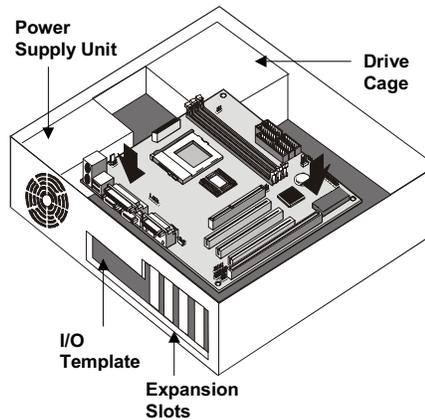
This illustration shows a mainboard installed in a tower-type case.
