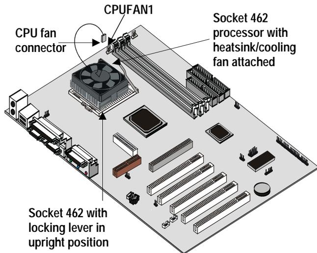
The mainboard must be configured to deliver the correct clock speed and the correct system bus for the kind of processor that you have installed. You can do this by using the BIOS Setup Utility. The first time you start the system, immediately enter the Setup Utility and make the appropriate settings. Usually, you can automatically configure the CPU by using the CPU & BIOS Features page of the Setup Utility. See Chapter 3 for more information.
