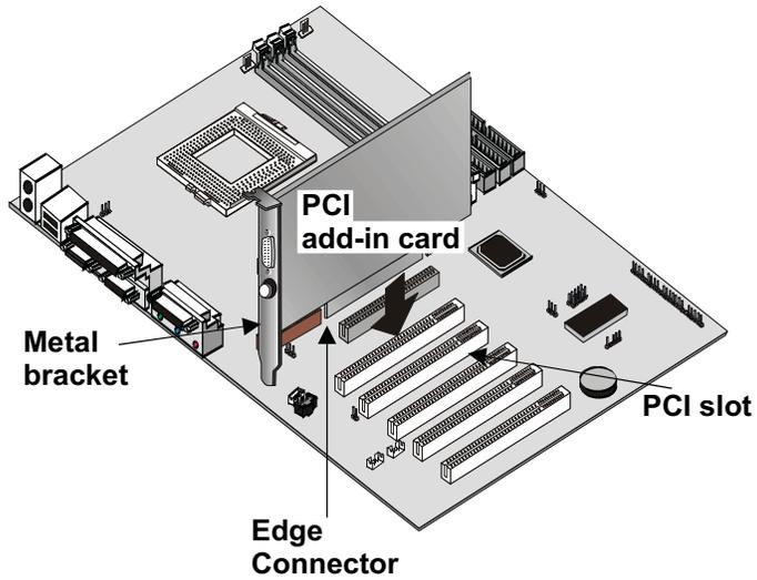
4. Secure the metal bracket of the card in the empty slot in the system case with a screw.
