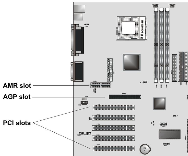
1. Before installing an add-in card, check the documentation for the card carefully. If the card is not Plug and Play, you may have to manually configure the card before installation.
