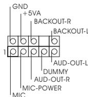
This is an interface for front panel audio cable that allows convenient connection and control of audio devices.
