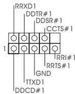
This connector supports a serial port module.
