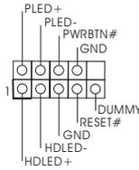
This connector accommodates several system front panel functions.
