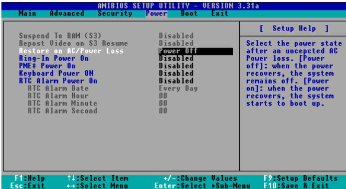
**Suspend to RAM (S3):** This field allows you to select whether to auto-detect or disable the ACPI Suspend-to-RAM feature. Select [Auto] will enable this feature if the system supports it.
