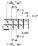
ASRock I/O™ already provided 4 default USB ports. If the 4 USB ports on the rear panel are not sufficient, an USB header is available for 2 additional USB ports.
