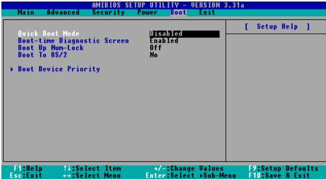
**Quick Boot Mode:** This mode speeds up the boot-up routine by skipping memory retestings.
