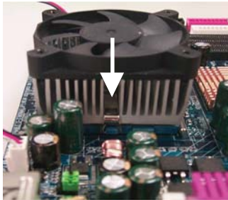
3. Fasten the heatsink supporting-base onto the CPU socket on the main-board.
