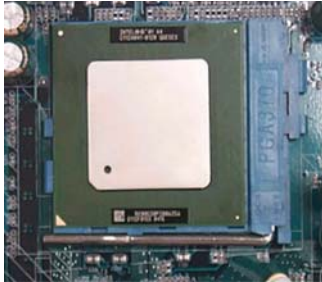
1. Press down the CPU socket lever and finish CPU installation.
