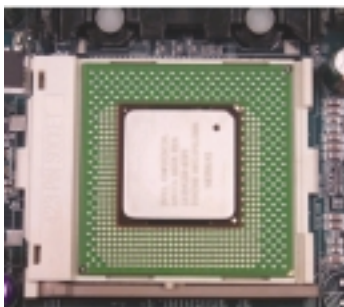
1. Align CPU and insert it
