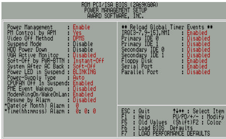
Figure 4.5: Power Management Setup
