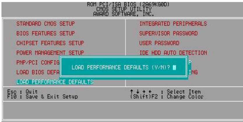
Figure 4.8: Load PERFORMANCE Defaults
