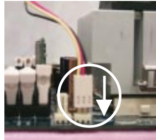
4. Make sure the CPU fan is plugged to the CPU fan connector, than install complete.
