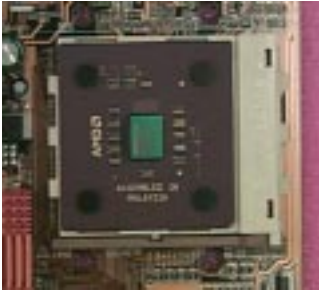
1. Press down the CPU socket lever and finish CPU installation.
