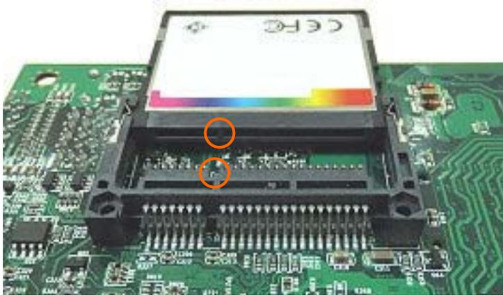
**Step 2:** Insert the CFAST card. Push the CFAST card in at a 180° angle.
