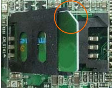
**Step5** : Flip down the cap, press down and slide the cap to the CLOSE position. Be sure that the cap is tightly held with the socket.
