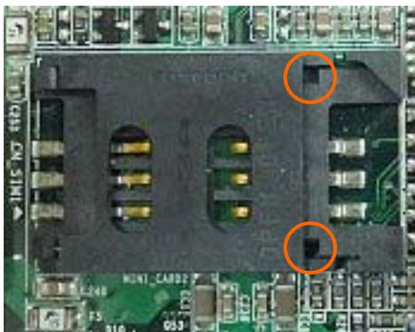
**Step3** : Flip the cap up for inserting a SIM card into.
