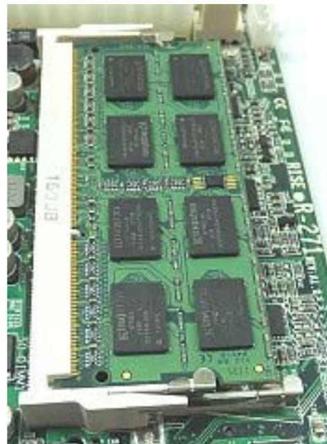
**Step 3:** Insert the SO-DIMM. Push the memory in at a 20° angle.
