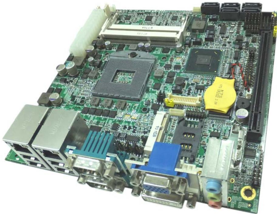
The R-271 series Mini-ITX motherboard is a Socket G 32nm Intel® Core™ i3, i5 and Core™ i7 processor platform. Up to two 8.0 GB 1066/1333/1600 MHz DDR3 SDRAM SO-DIMM are supported by the Intel® processor. The processor also supports a PCIe x16 slot.
