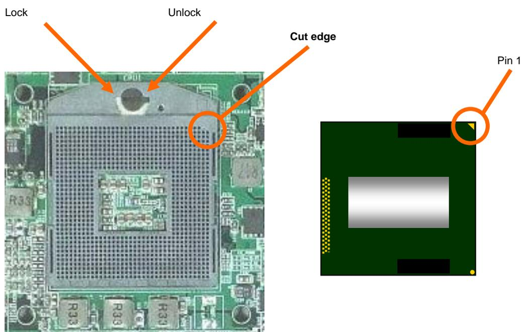
**Step 2 :** Inspect the CPU socket. Make sure there are no bent pins and make sure the socket contacts are free of foreign material. If any debris is found, remove it with compressed air.
