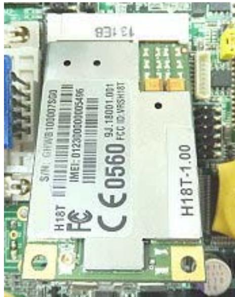
**Step 2:** Seat the MINI PCI-E card. Gently push downwards and the arms clip into place.
