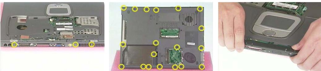
4. Remove the two screws. Then take the right and the left antenna off the main unit.
