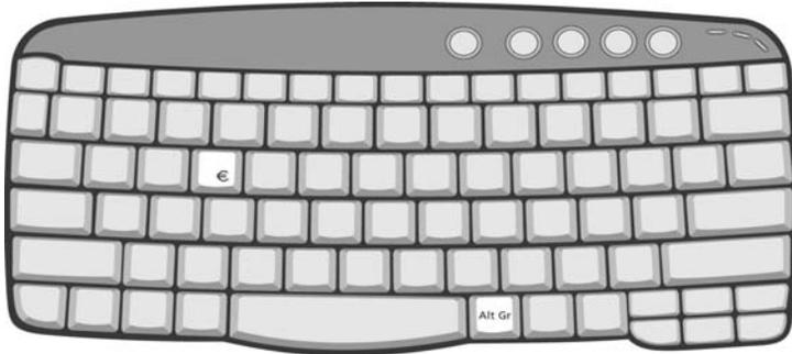
**NOTE:** For US keyboard users: The keyboard layout is set when you first set up Windows. For the Euro symbol to work, the keyboard layout has to be set to United States-International.
