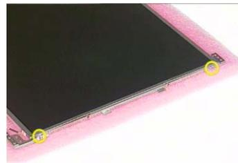
7. Tear off the electric conductive tape that fastens the LCD coaxial cable.
