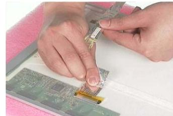
10. Detach the wireless antenna from the LCD panel.
