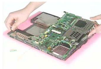
11. Unscrew the two screws that fasten the HDD bracket.
