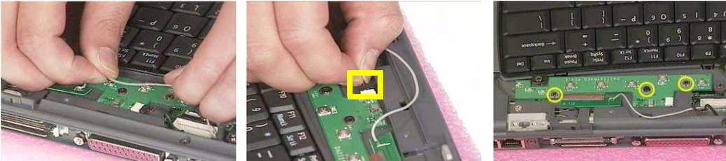
4. Remove the three screws that secure the keyboard.
