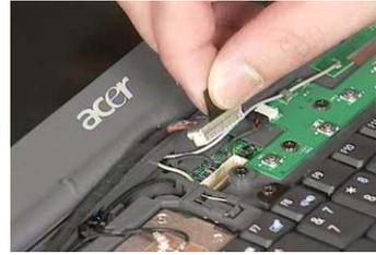
4. Disconnect the left bluetooth antenna line. Then take out the antenna from the upper case with a tweezers.
