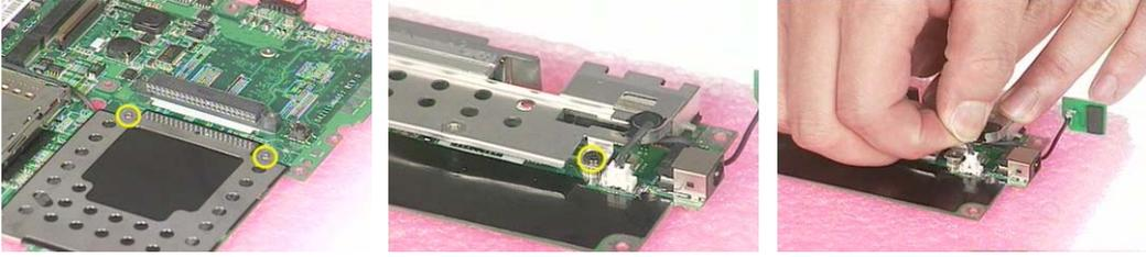
14. Turn the CPU lock counter clock-wise with a flat head screw driver. Then remove the CPU.
