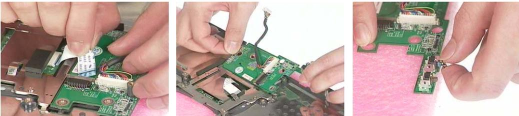
6. Remove the four screws that fasten the touchpad holder.
