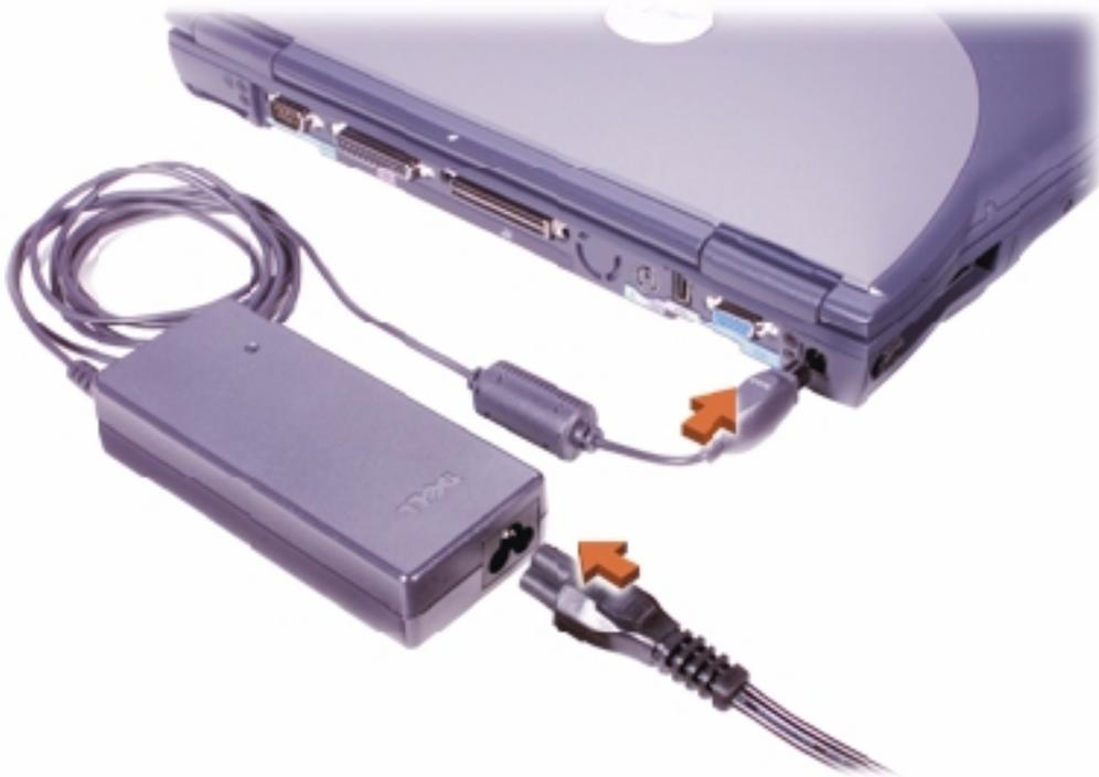
The AC adapter converts AC power to the DC power required by the computer. You can connect the AC adapter with your computer turned either on or off.
