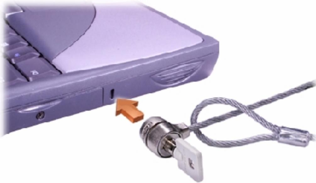
This slot allows you to attach a commercially available antitheft device to the computer. Instructions for installing antitheft devices are usually included with the device.
