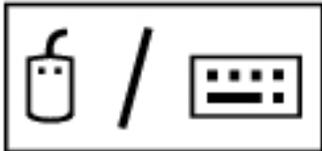
Use this connector to attach PS/2-compatible devices, such as a mouse, keyboard, or external numeric keypad.
