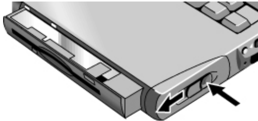
Figure 2-3. Removing a Module
