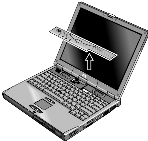
Figure 2-9. Removing the Power Button Panel
